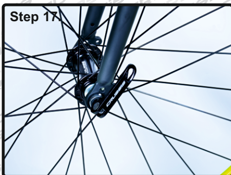
Correct position of the quick release axle to the fork after tightening
