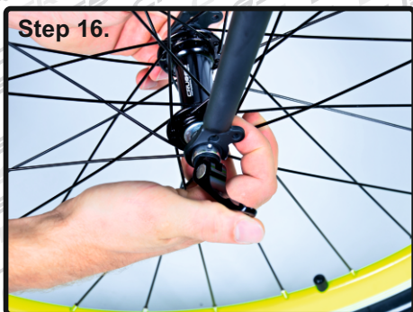
Tighten quick release. Mind the direction of the wheel
