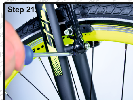
If the brake is rubbing the rim adjust the position of the brake pad. With tightening the screw distance will increase
