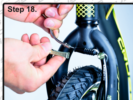
At the front and rear brake put cable guard into cable bridge
