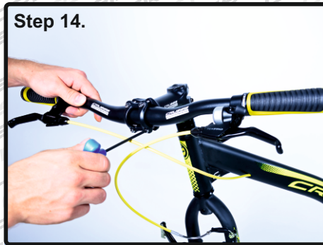
Put back the front part of the stem and lightly tighten, adjust the angle of the handlebar and screw it with 4 NM
