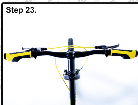
Stem and front wheel must form a single axis. Make sure that stem is properly tightened with force 4 NM
